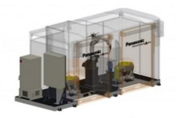
The Panasonic arc welding robot cell PERFORMARC TT (Table-Table) is of a modular concept, developed using standard reliable Panasonic components.
