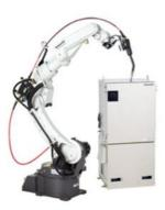
This welding robot series features an externally or internally mounted torch cable, and a high resolution encoder with a highly rigid arm.
