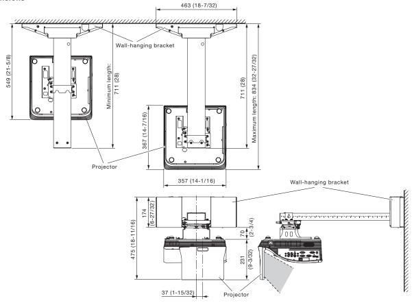
The illustration shows the wall-hanging bracket attached to the projector.
