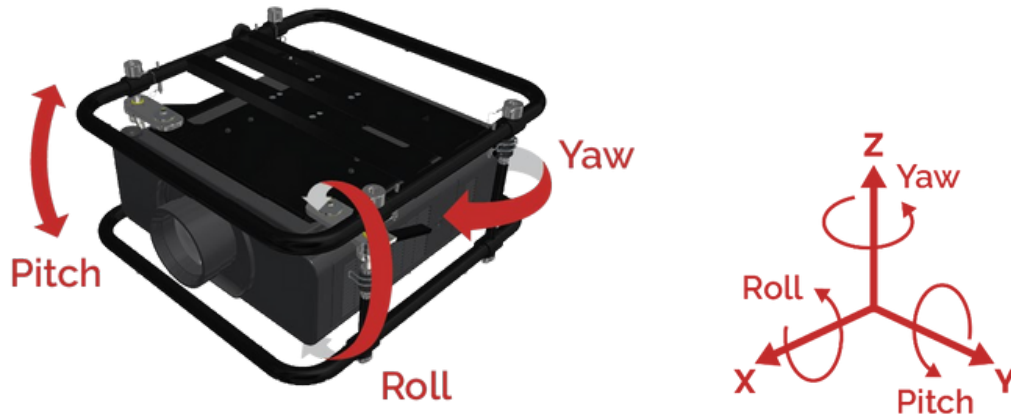
Figure 16 Illustration of yaw, pitch and roll
