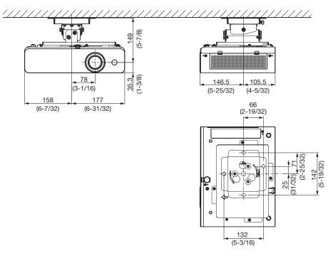
The illustration shows the ceiling mount bracket when it is combined with the ET-PKL430B and the PT-TW341R/TW340/TW250/TX400/TX310/TX210 is attached.
