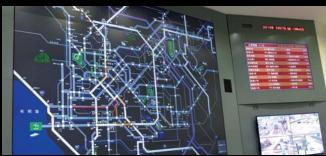
Huge screen surface area is enabled with five sets of four PT-RZ670 projectors displaying 72-inch images at 16:10 aspect.
