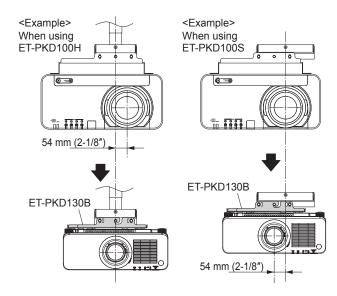
center of the attachment plate. However, when replaced with PT-DZ870, for example, the center position will shift to the left by 54 mm (2-1/8") as shown in the figure on the right.
