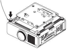
3) Turn the adjustment leg clockwise to secure it to the projector.
