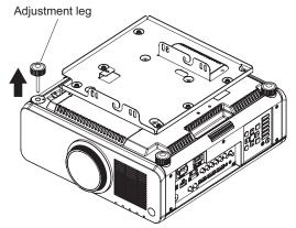
1) Turn the adjustment leg (one) counterclockwise to remove it from the projector.
