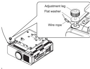
2) Pass the supplied flat washer (one) and wire rope through the adjustment leg (one) as illustrated on the left.
