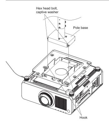
2) Fit the finger tightened captive washer hex head bolts in the pole base (the attachment plate for a ceiling mount bracket for low ceilings) in the hooks on the angle adjusting bracket.
