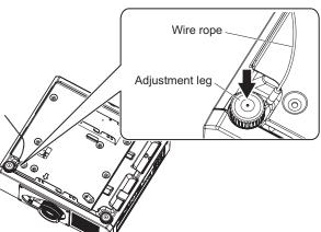
When attaching the wire rope to a group F projector, pull out the wire rope as illustrated on the left, and tighten the adjustment leg.
