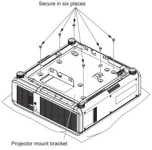
3) Firmly secure the projector mount bracket to the bottom of the projector using the six supplied captive washer hex head bolts (M6 × 16) as shown in the figure on the left.
