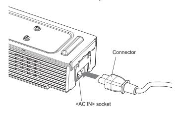
Check the shapes of the <AC IN> socket of the projector and the connector of the power cord and then orient the connector correctly and insert it firmly.
