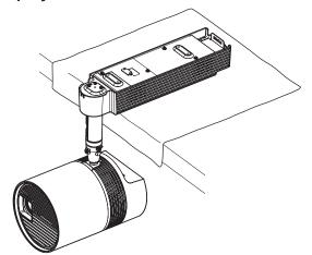
Prepare a bench for the mounting work with a height of at least 280 mm (11") and lay a soft cloth or the like below the projector to prevent scratches.
