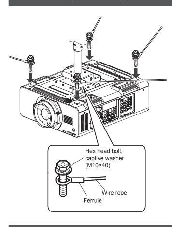
2) As shown in the figure on the left, pass the supplied hex head bolts with washers (M10 × 40) through the rings in the supplied wire rope, and secure the bolts to the threaded holes in which the adjustable feet were previously attached.
