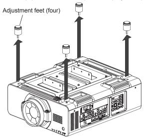
1) Turn the adjustable feet (four) counterclockwise to remove it from the projector.
