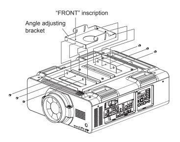
Secure the angle adjusting bracket to the projector mount bracket using the six supplied captive washer screws (M6 x 16) as illustrated on the left.
