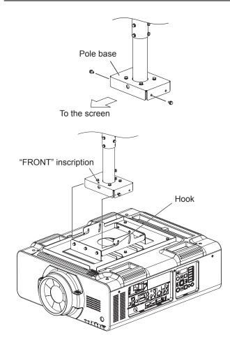
Temporarily secure two of the supplied captive washer hex head bolts (M8×20) to the front screw holes ("FRONT" inscription) on the left and right sides of the pole base.
