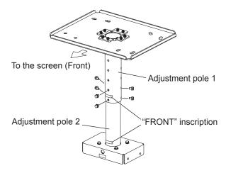
Insert the adjustment pole 1 into the adjustment pole 2, align the holes, and secure them with the supplied six captive washer hex head bolts ( $M6 \times 16$ ).
