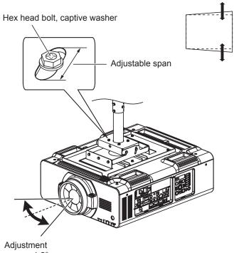
the pole base and then swivel the projector head horizontally until the picture is centered on the screen.Once the picture position has been set, be sure to
