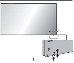
Slide the lever on the rear panel to eject the power indicator and remote control sensor.
