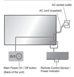
Operate pointing the remote control directly at the unit's Remote Control Sensor.
