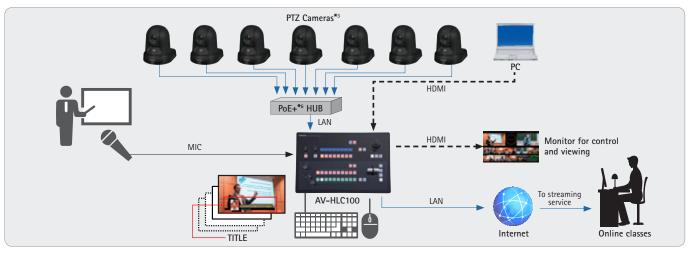
\*1: A PoE+ hub is required for the power supply. \*2: See "Supported Formats" on page 5 for details. \*3: NDI® / NDI® | HX compatible models. See the Panasonic website for Panasonic Integrated Cameras compatible with NDI® / NDI® | HX (https://pro-av.panasonic.net/en/products/ptz\_camera\_systems.html ). \*4: Abbreviation of Power over Ethernet Plus Plus. \*5: See "Supported Formats" on page 6 for details. \*6: Abbreviation of Power over Ethernet Plus.
