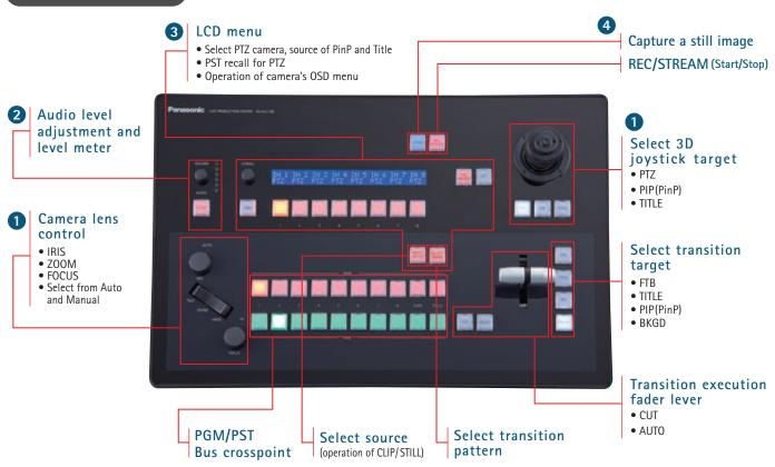
The extremely user-friendly panel includes buttons for various functions including camera control and switching, along with audio mixing. Up to eight video systems can be freely assigned to the crosspoint buttons, enabling them to be selected easily. With the capability to handle IP input and output, the AV-HLC100 also allows for live streaming and recording all over IP.
