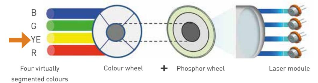
Not only does this make the colour more balanced it also contributes to a higher perceived brightness as the brightness output per colour channel is significantly increased. Another reason why the Panasonic 6500 lm laser projector can perform well against projectors of a higher brightness category.
