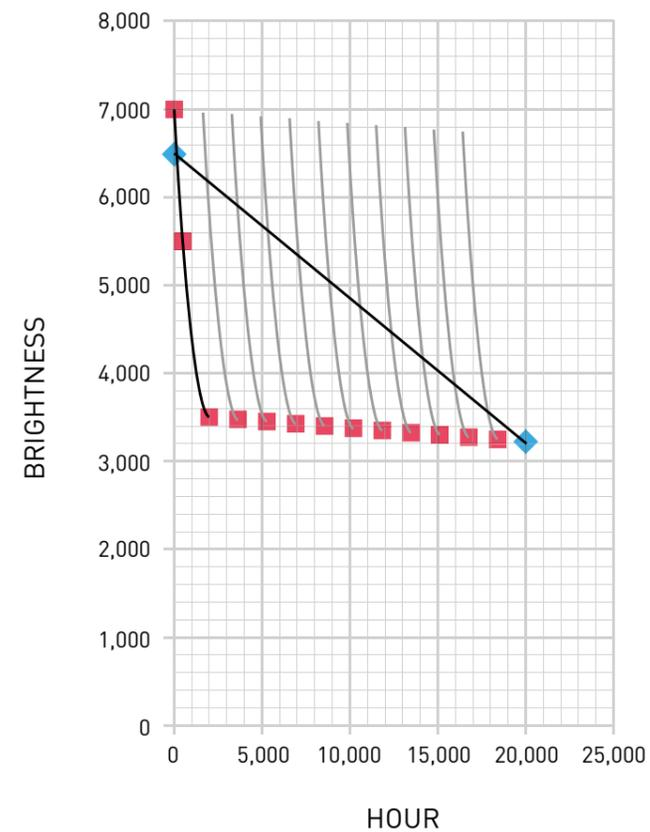
Where we compare the performance of a conventional projector rated at 7,000 lm against that of a Solid Shine model rated at 6,500 lm it can be seen that, because of the **Regressive Decay** pattern of the lamp-lit projector, after only a short period of use, the Solid Shine model is operating at a superior level of brightness. In the attached graphic, the brightness of the lamp-lit 7,000 lm projector falls below that of the Panasonic 6500 lm laser projector after just 159 hours of use.
