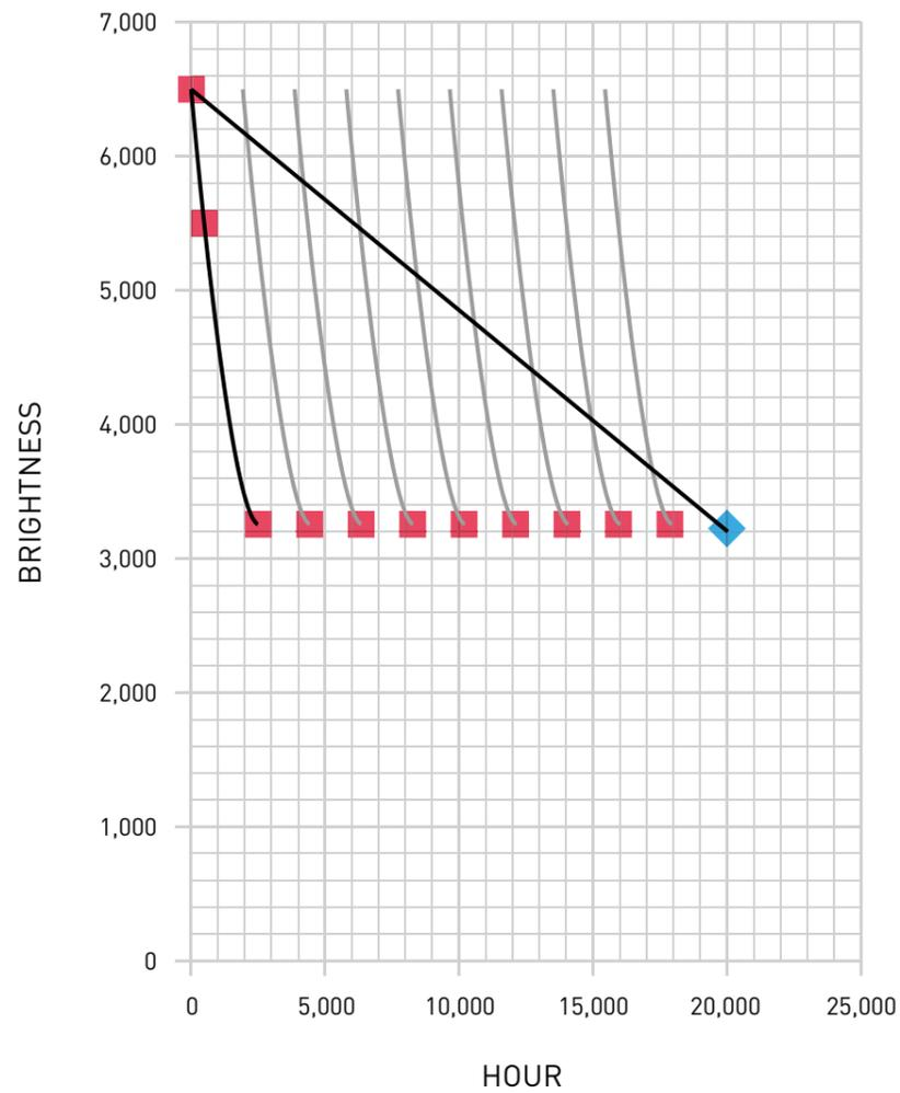
The graph opposite shows the brightness output of two projectors, both with an initial rating of 6,500 lm: one a conventional lamp-lit projector, the other a laser projector. It can be seen that the brightness of the lamp-lit model rapidly falls below the Solid Shine model. Even after an expensive bulb change, the conventional model matches the performance of the Solid Shine model only for a short time.
