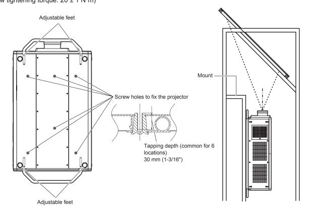
Position of screw holes to fix projector and adjustable feet
