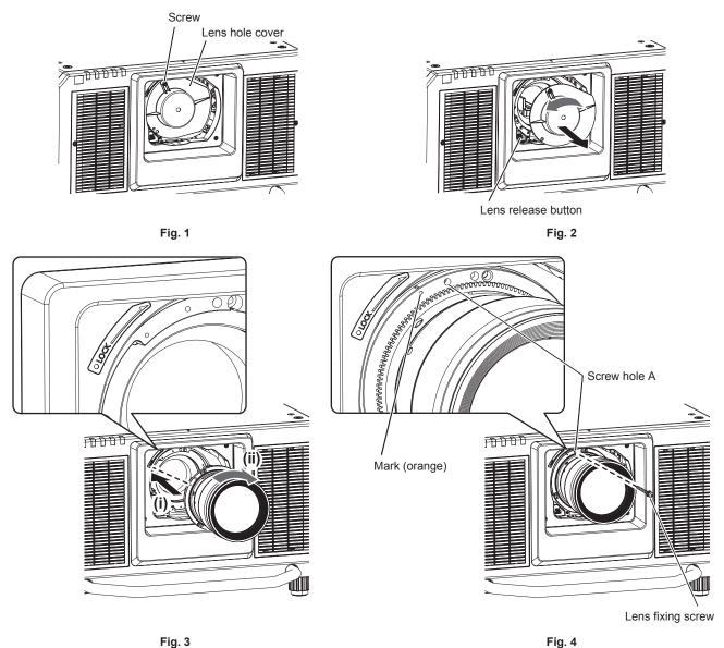
1) Loosen the screw fixing the lens hole cover. (Fig. 1)
