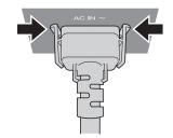
1) Check the shapes of the <AC IN> terminal on the side of the projector and the power cord connector, and insert the connector completely in the correct direction (until you hear the side tabs click in place).
