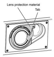
1) Hold the tab of the lens protection material and remove the lens protection material by pulling in the direction of the arrow.
