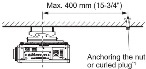
1) Mount the anchoring nut or curled plug (M8) in the concrete ceiling (at a single point within the area shown in the diagram on the left).
