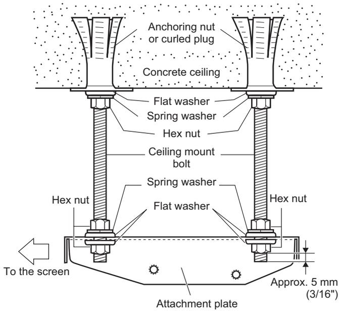
1) Attach the anchoring nuts or curled plugs to a concrete ceiling and securely fix the four ceiling mount bolts. (Refer to page 6 for attachment positions.)
