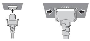
1) Check the shapes of the <AC IN> terminal on the rear of the projector body and the power cord connector, and insert the plug completely in the correct direction (until you hear the side tabs click in place).
