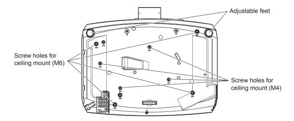
The positions of screw holes for ceiling mount and adjustable feet
