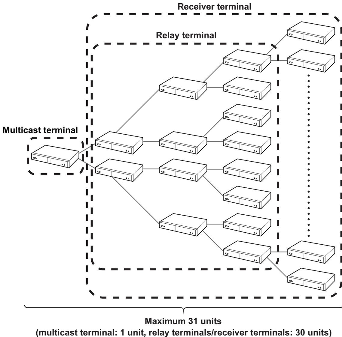
The multicast feature, compared to usage of an MCU, can reduce the network bandwidth used at the multicast terminal's sites. When a transmission failure occurs during the multicast, the configuration of the terminals will automatically change, so it is necessary that all terminals can connect and communicate with each other over the network.
