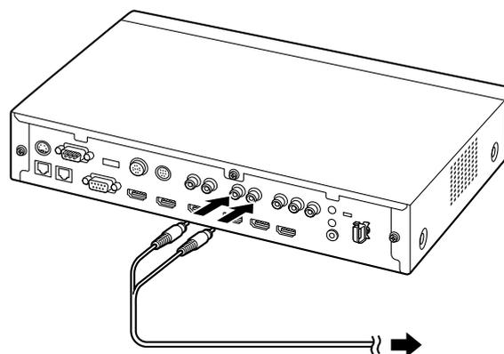
1. Connect the amplifier/active speaker to the Audio Out L/R jack on the back of the unit using a stereo pin plug cable.
