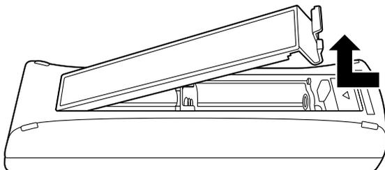
2. Insert batteries (R6/LR6 [AA] dry cell<sup>\*1</sup>), minus side first, then close the cover.
