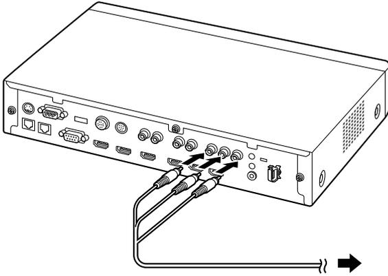
1. Connect the display to the Component terminal on the back of the unit using a component cable.
