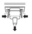
Unplug the connector pressing the two knobs.
