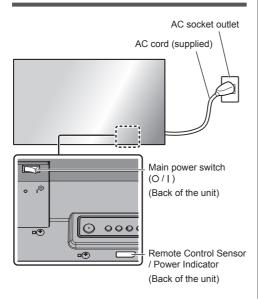
Operate pointing the remote control directly at the unit's Remote Control Sensor.
