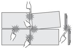
When multiple displays are installed, a material to protect the top face of the LCD panel has been attached on the top face of this unit. When installing multiple displays, extend this protection material toward the display surface side. After installing multiple displays, cut off this protection material from the cutting-off line, and then adjust the gaps.
