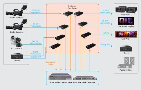
\*Deltacast FLEX modules are required for baseband input/output.
