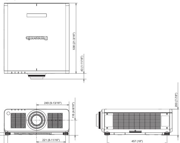
\* The above dimensions are obtained when the standard zoom lens is attached. \* Actual dimensions may differ depending on the product.
