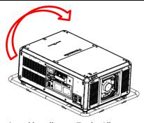
2)Remove the screw that secures the main unit and handle. M6 hexagon socket head cap screw 16pieces.
