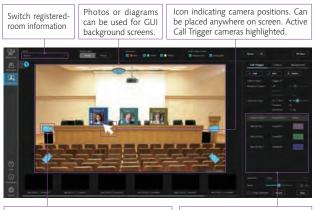
Call Trigger icon recalls presets of associated cameras with one click. Note:Two-step preset recall possible.
