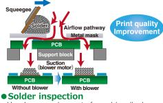
Head camera inspects for solder displacement, bridging, streaking, and bleeding.
