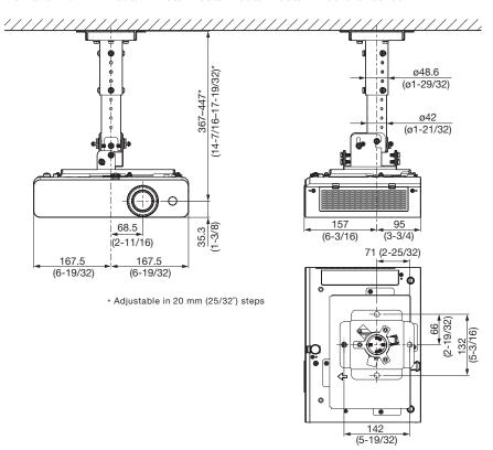
The illustration shows the ceiling mount bracket when it is combined with the ET-PKL430B and the PT-TW341R/TW340/TW250/TX400/TX310/TX210 is attached.
