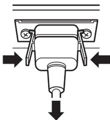
Unplug the connector pressing the two knobs.
