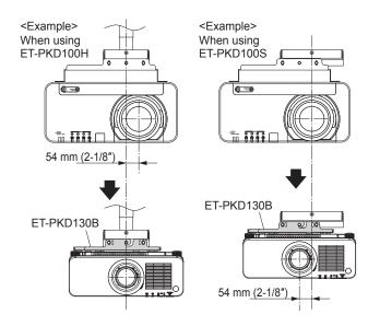
center of the attachment plate. However, when replaced with PT-DZ870, for example, the center position will shift to the left by 54 mm (2-1/8") as shown in the figure on the right.
