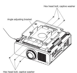
Align the screw holes on the angle adjusting bracket with the holes on the projector mount bracket and secure the bracket with the six captive washer hex head bolts removed in the section "Removing the projector from the existing bracket", as shown in the figure on the left.
