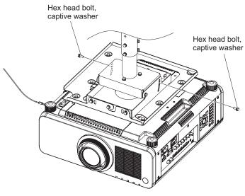
3) Use the two captive washer hex head bolts removed in the section "Removing the projector from the existing bracket" to secure the pole base (the attachment plate for a ceiling bracket for low ceilings) and the angle adjusting bracket as shown in the figure on the left.
