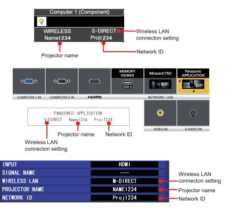
If the input guidance does not appear, press the <MENU> button of the projector, and on the menu that is now displayed, select [DISPLAY OPTION] → [INPUT GUIDE] → "ON" or "DETAILED".
