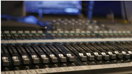
The 32-channel mixing desk provides control for the whole auditorium, including the Panasonic projector.
