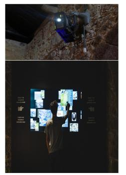
The full system consists of equipment from six Panasonic models. 10 PT-RZ970 laser projectors, which are outstanding for their durability, allow the museum to remain open all day long. There are also PT- RZ670 and PT-RZ470 projectors, both chosen from a compact range which produces surprisingly bright images. They deliver a powerful visual effect.
