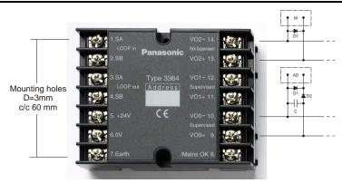
**VO0 & VO1**: **AD**=Alarm Device (bell, siren, etc.). **VO2**: **M**=Fire door release magnet(s). **D1**=Suppression diode (1N4004), when required. **D2**=Series diode (1N4004). **C** (470nF, supplied), to be connected in the last device <u>or</u> in up to five devices.
