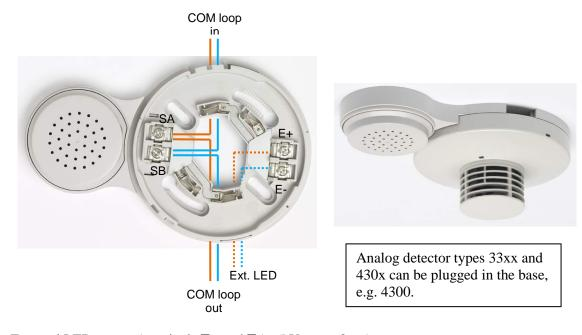
External LED output (terminals **E**+ and **E**-): 5 V, max. 2 mA. One External indicator (LED), e.g. 2218, can be connected to the base.
