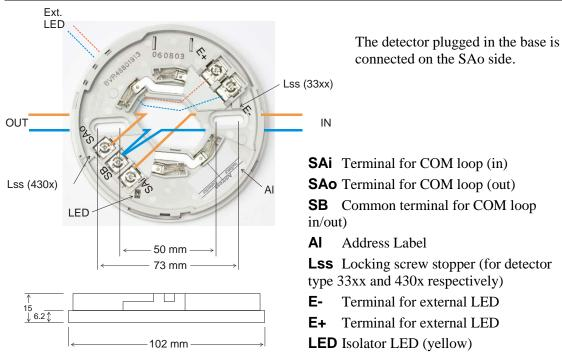
Isolator LED: Normal state = one blink 250 ms / 3 s. Isolated state = two blinks 250 ms / 3 s. NOTE! The LED is not visible when the detector is plugged in the base.
