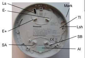
The detector is plugged in the analog base 3312x / 4313. The COM loop / Ext. LED are connected to the analog base.
