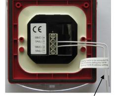
Flying leads to be connected to the Address setting tool 3314 during mode and address setting
