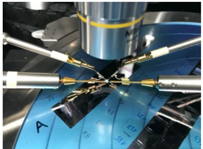
Figure 7: Electrodes for resistance measurement
