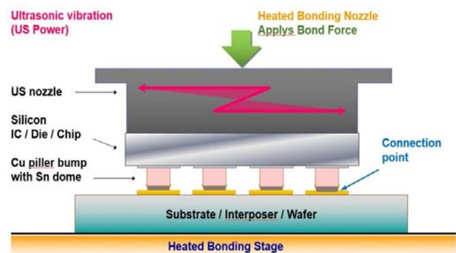
Figure 1: Schematic drawing of Thermo-Sonic Flip-chip Bonder
