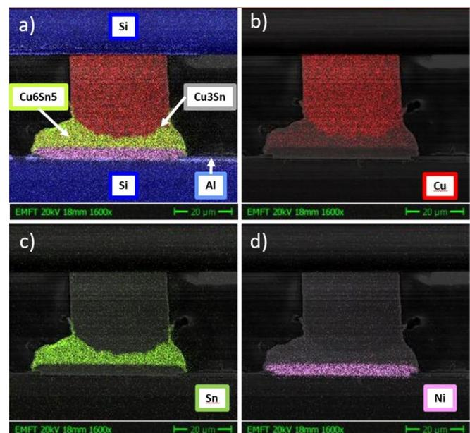
Figure 9: (a) EDX color mapping of Cu-SnAg-Au interconnection after TS-FCB and gang bonding. Single elements: (b) Cu, (c) Sn and (d) Ni
