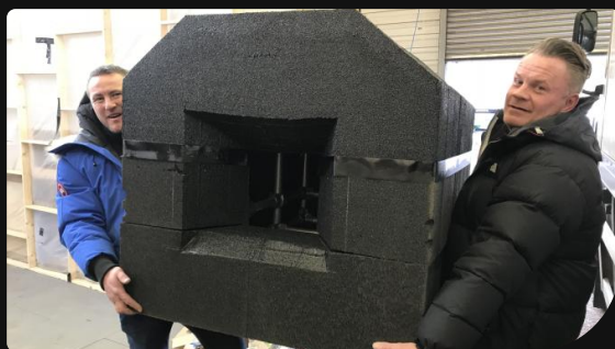
Crash box made for the VariCam LT for the lake sequence
