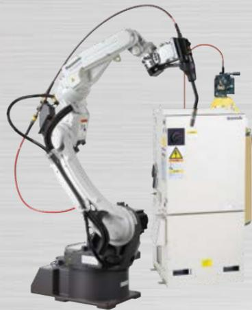
The new Super Active torch with air cooling mechanism increases the duty cycle and allows use in higher current ranges.
