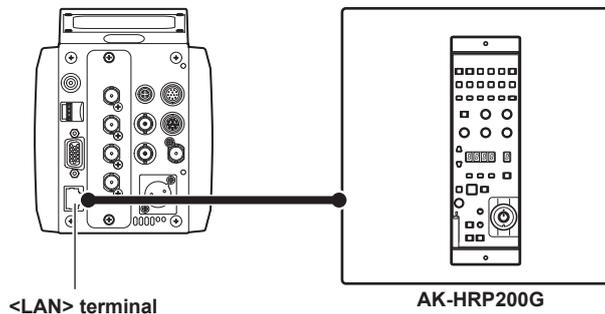
**1** Connect the <LAN> terminal of this camera to the <LAN> terminal of the remote operation panel AK-HRP200G.
