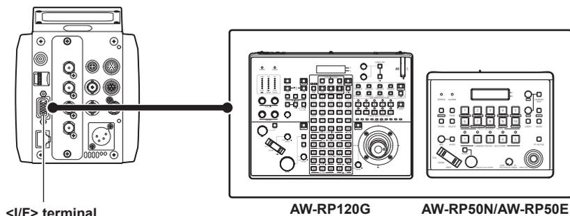
**1** Connect the <I/F> terminal of this unit to the <TO PAN/TILT HEAD> terminal of the remote camera controller AW-RP50N/AW-RP50E/AW-RP120G.
