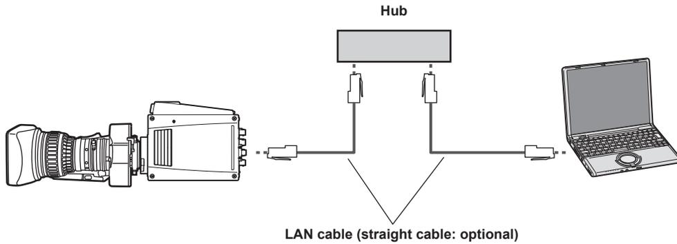
Set the IP address of the personal computer with a separate address of AK-UB300G within the range of private address.
