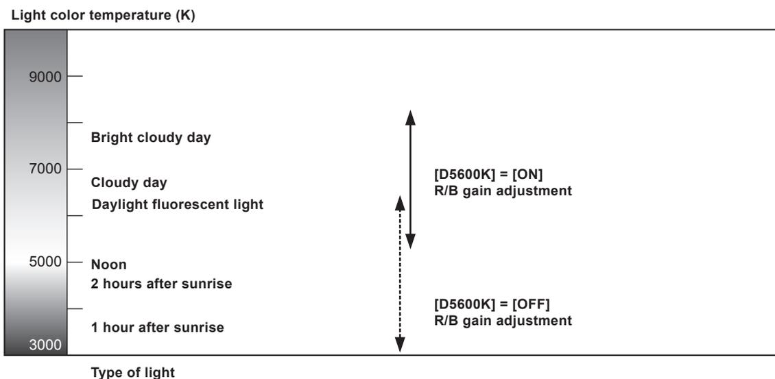
Color temperature is automatically adjusted by controlling the R and B gains with the [OFF] or [ON] setting value in [D5600K].
