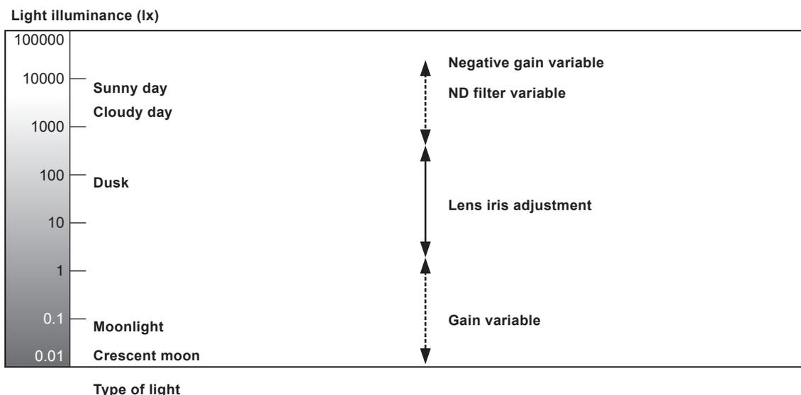
Automatic adjustment is performed by controlling the lens aperture, gain (including frame addition), ND filter, and negative gain.
