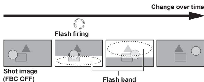
The flash band compensation function is enabled when set to [MAIN MENU] → [SWITCH MODE] → [FBC SETTING] → [FBC] → [ON]. The flash strobe light such as a still camera is detected and can be compensated.
