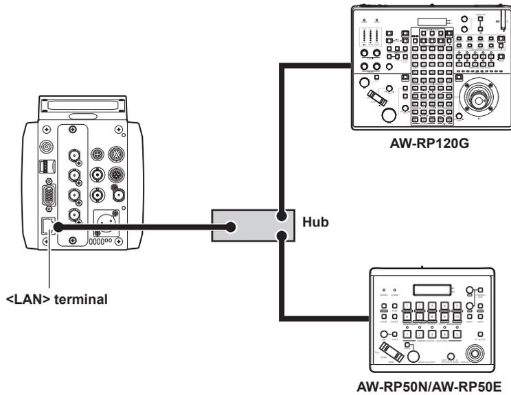
**1** Connect the <LAN> terminal of this unit to the <LAN> terminal of the remote camera controller AW-RP50N/AW-RP50E/ AW-RP120G.
