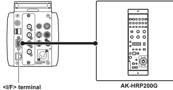
**1** Connect the <I/F> terminal of this camera to the <RS-422> terminal of the remote operation panel AK-HRP200G.
