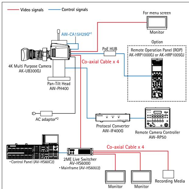
\*1: AW-CA15H29G is not required when a remote operation panel (ROP) is directly connected to AK-UB300GJ. \*2: 60 W or more is recommended.
