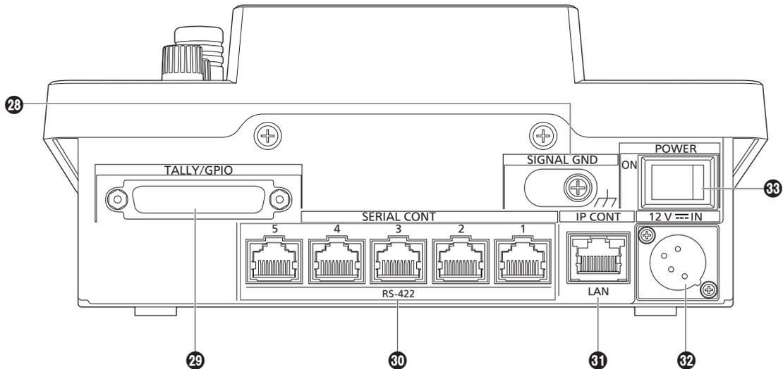
**28 Grounding terminal [SIGNAL GND]**
