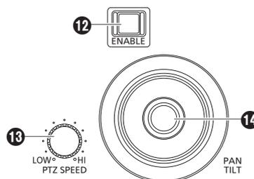
12 PAN/TILT / IRIS / ZOOM / FOCUS ENABLE button [ENABLE]
