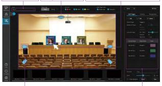
Call Trigger icon recalls presets of associated cameras with one click. Note:Two-step preset recall possible.
