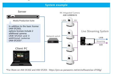
Using AW-SF100 to manage operations at a classroom Auto tracking and control of one camera with one PC
