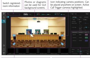
Call Trigger icon recalls presets of associated cameras with one click. Note:Two-step preset recall possible.
