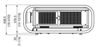
Illustration shows the frame attached to PT-RQ22K/RZ21K/RS20K.
