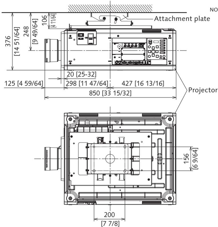
The illustration shows the ET-PKD520H ceiling mount bracket mounted on Group C projectors (PT-RQ13K/PT-RZ12K/PT-RS11K)
