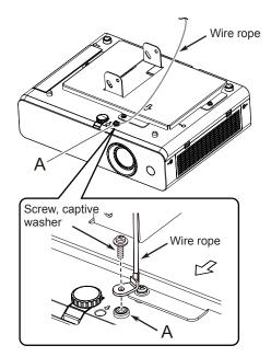
As shown in the figure on the left, secure the one end (round crimping terminal) of the supplied wire rope to the A on the projector by using the 1 supplied captive washer screw (M4 x 12).
