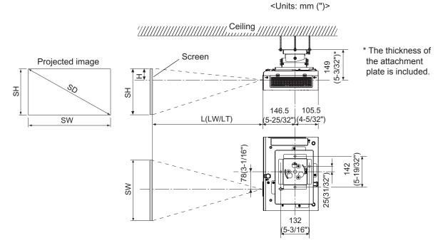
(When using the ceiling mount bracket ET-PKL100H (for high ceilings))
