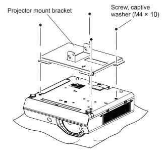
3 Secure the projector mount bracket to the bottom of the projector using the 4 supplied captive washer screws (M4 × 10) as illustrated on the left.
