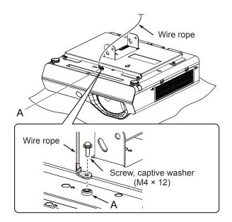
As shown in the figure on the left, secure the one end (round crimping terminal) of the supplied wire rope to the A on the projector by using the 1 supplied captive washer screw (M4  $\times$  12).
