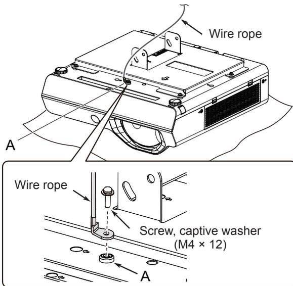
As shown in the figure on the left, secure the one end (round crimping terminal) of the supplied wire rope to the A on the projector by using the 1 supplied captive washer screw (M4 x 12).
