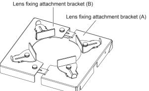
5) Separate lens fixing attachment bracket (A) and lens fixing attachment bracket (B) as shown in the figure.
