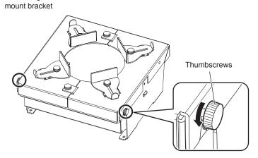
2) Loosen the two lower thumbscrews (inserted in slots).
