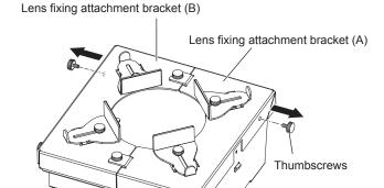
1) Remove the two upper thumbscrews (inserted in round holes).
