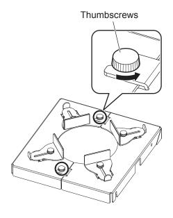
4) Loosen the thumbscrews (two places) at the center of the lens fixing attachment bracket.
