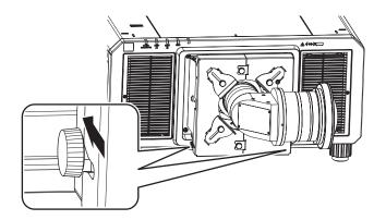
5) Attach the lens fixing attachment bracket to the lens fixing attachment mount bracket as shown in the figure.
