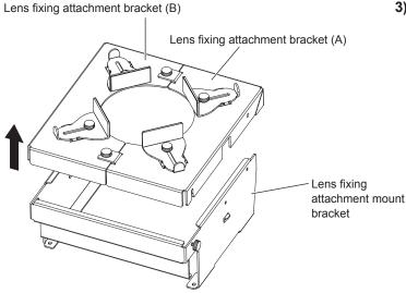
3) Remove the lens fixing attachment bracket as shown in the figure.
